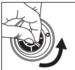
To replace the filter, remove the bottle cap, rotate the filter in an anti-clockwise direction and remove it by pulling it upwards.
